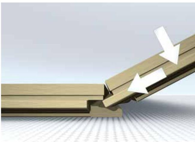
Hold the panel to be installed at an angle of 20° to 30°. Move the panel gently up and down and at the same time exert forward pressure. The panels will automatically click into place.
