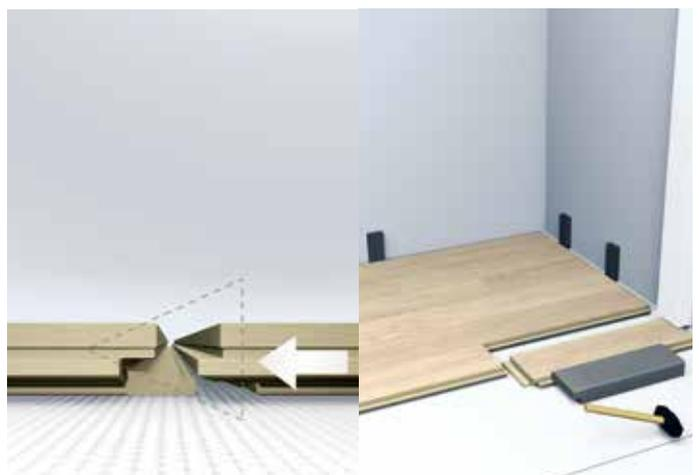
Ideal for awkward corners or installing under door frames. Unlike most other systems, Uniclic® panels can also be joined together horizontally. This is essential when you install the last row of panels to be installed or in places where it is difficult or even impossible to rotate the panels (underneath door frames, for example).
